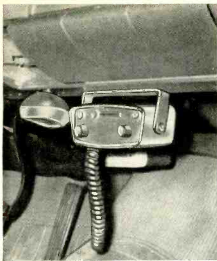
Fig. 5—Control head and mike are mounted in center or slightly left-center on the dash.
