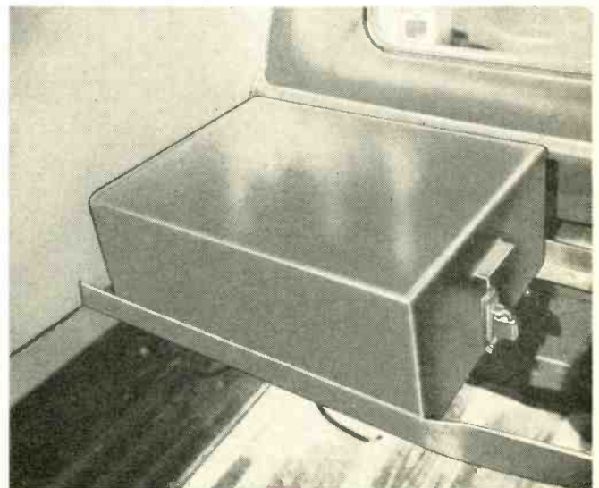
Fig. 2 —Weatherproof housing is made of sheet metal. Lock keeps the public out.
