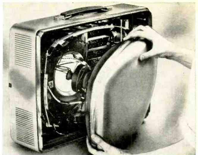
In the new RCA portable, picture tube can be easily removed from front of set.
