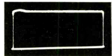
Fig. 5—Basic test setup to check 300-ohm rf impedance: a—300-ohm delay line about 5 feet long can be used to check tuner input impedance: b—If input impedance is 300 ohms, a practically flat trace is obtained on an rf sweep test.
